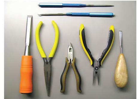
Figure 16: Remove supports using the proper tools such as a chisel, magnetic handle pick set, pliers, and needle nose pliers.
